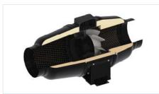
Due to the conic impeller and special blade profiling the circumferential air speed increases thus providing higher air pressure and capacity as compared to standard axial fans. The diffuser, the specially profiled impeller and the directing vanes at outlet from the fan casing distribute air flow in such a way as to attain the best combination of high performance and high pressure at low noise level. The fan casing is equipped with an airtight terminal box for connection to power mains.
